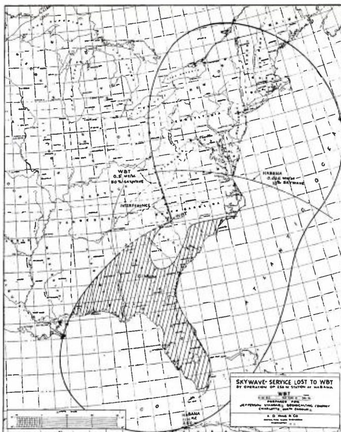
ONE of the clinchers in the U. S. industry advisory delegation's decision against acceptance of Cuban NARBA proposals was this map, showing in shaded areas the skywave losses WBT Charlotte would suffer from proposed 250-w Havana co-channel station. Havana station's service radius would be about two miles.
